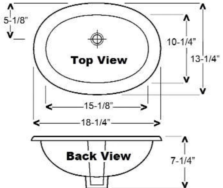
Dimensions of fixture are nominal and may vary within the range of tolerances established by ASME Standard A112.19.2.2018. Dimensions and specifications subject to change without notice.
