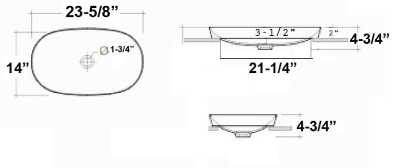
Dimensions of fixture are nominal and may vary within the range of tolerances established by ASME Standard A112.19.2.2018. Dimensions and specifications subject to change without notice.
